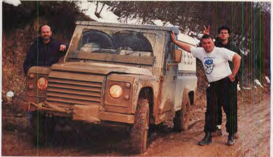
Tony Gathercole, British forces vet, with armored Land-Rover on central Bosnia's "Ho Chi Minh Trail." Tony's firm, TEAM Armored Vehicles, is leasing and maintaining press vehicles in Bosnia. This Rover has steel armor and heavy glass protecting cab only against 7.62 caliber rifle fire. Counter-mine plate — about three-eighths-inch thick steel — is bolted underneath. Reuters team in similar vehicle survived mine blast in January with only broken legs and back injuries. Photo: courtesy Tony Gathercole
